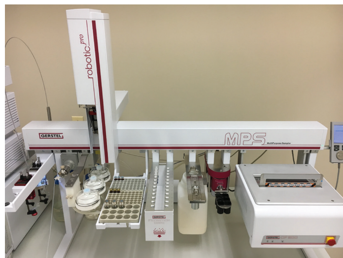
Figure 1: MPS robotic PRO Multi-Purpose Sampler with the GERSTEL QuickMix, CF-200 centrifuge, and Universal Filtration option.
