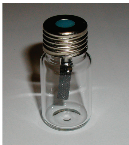
Figure 1: TF-SPME device in 10 mL vial.
