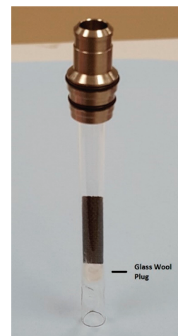
Figure 2: TF-SPME device in TDU tube.
