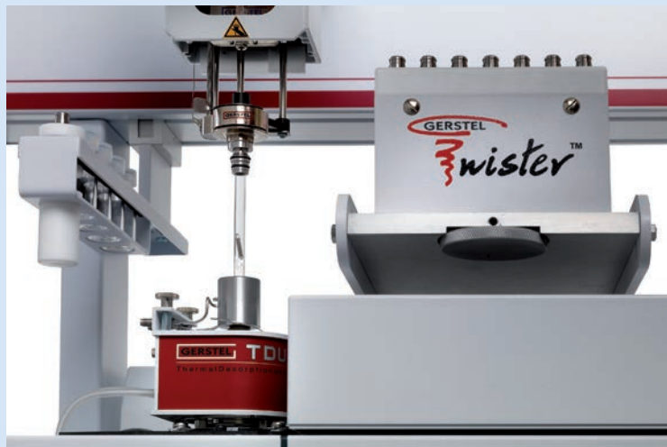
Stir Bar Sorptive Extraction using the GERSTEL Twister is followed by thermal desorption in the Thermal Desorption Unit (TDU), cryofocusing, and GC/MS analysis – fully automated using the GERSTEL MultiPurpose Sampler (MPS) under MAESTRO control.
