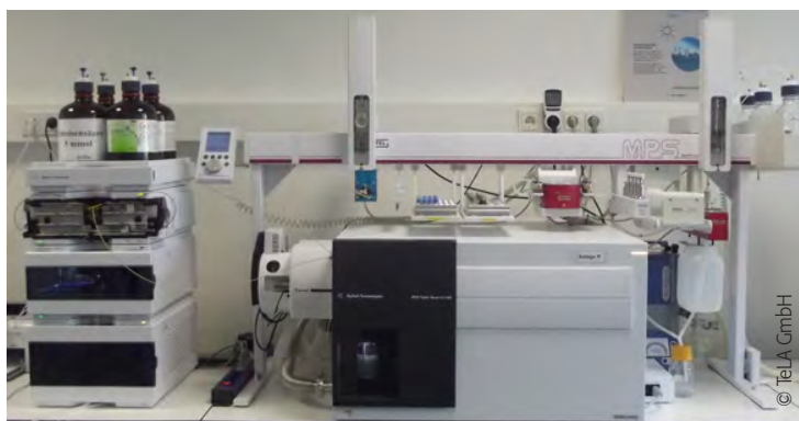
Instrument setup used for the automated determination of pyrrolizidine alkaloids: GERSTEL MultiPurpose Sampler (MPS) configured for automated SPE in combination with an LC-MS/MS system from Agilent Technologies (1290 HPLC and 6495 Triple Quadrupole LC/MS).
