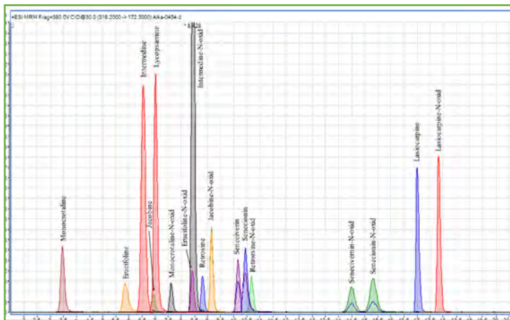
Analysis of a standard mixture of 17 pyrrolizidine alkaloids resulted in a clean chromatogram with well resolved peaks. Good separation of the individual PA compounds is extremely important. Many exhibit very similar mass transitions and can only be distinguished and identified unequivocally when peaks are fully resolved. (Source: TeLA GmbH)
