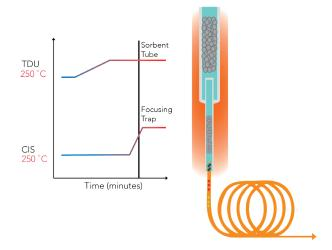
As the heaviest compounds reach the trap, it is rapidly heated so all compounds reach the head of the gas chromatographic column at once. This ensures optimum separation with the lowest detection limits.
