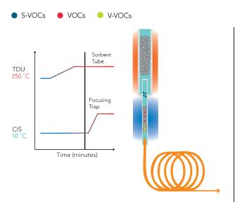
In this method, the Thermal Desorption tube is gradually heated to release S-VOCs, VOCs, and V-VOCs on to a high-capacity focusing trap that is kept cool.
