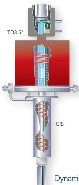
The TD 3.5+ is coupled directly to the Cooled Injection System (CIS): The "Liner-in-Liner" design ensures best possible analyte transfer to the GC column without discrimination or cross contamination. The built in TD 3.5+ alignment support simplifies liner replacement and mounting.
