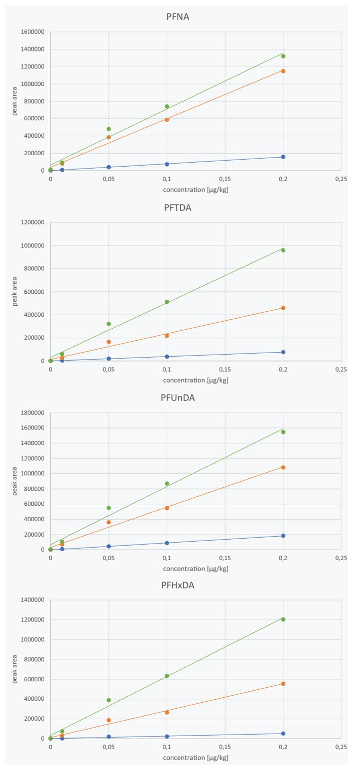
**Figure 6:** Comparison of peak area versus concentration (calibration) curves for selected compounds in egg obtained with online SPE and cartridge wash (green), online SPE without cartridge wash (orange) and direct injection (blue), respectively.
