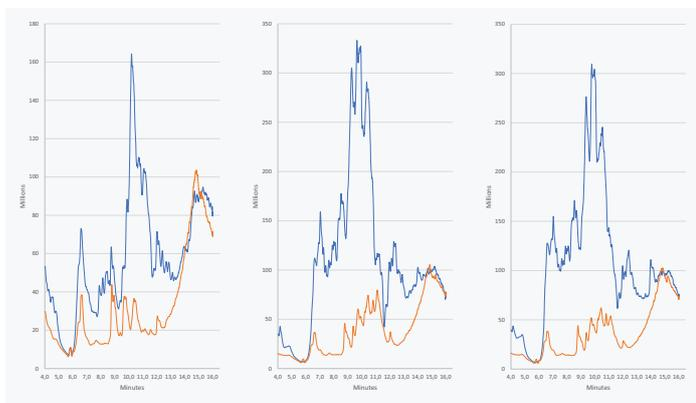
**Figure 4:** Comparison of total ion current chromatograms resulting from online SPE-LC-MS/MS analysis without and with cartridge wash for egg, fish and meat (from left to right).
