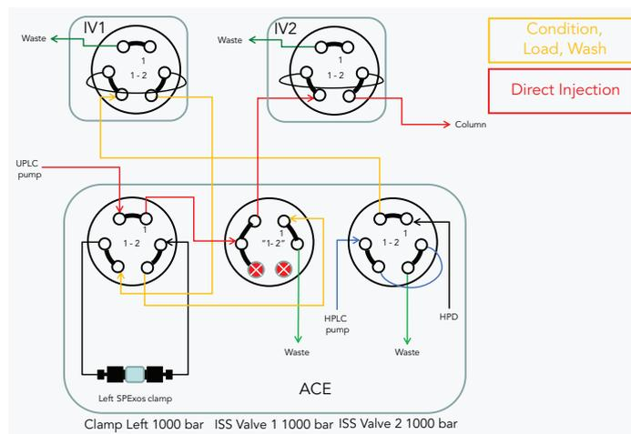
**Figure 2:** Flow path during conditioning, load, and wash of the cartridge. The same valve positions allow direct injection to LC/MS through injection valve IV2.
