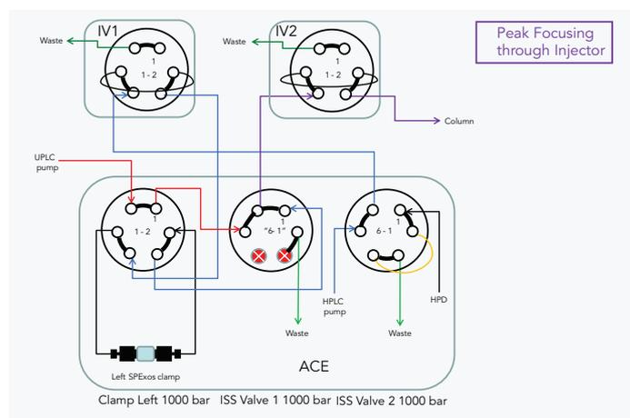
**Figure 3:** Flow path during elution of the cartridge with peak focusing on the LC column.
