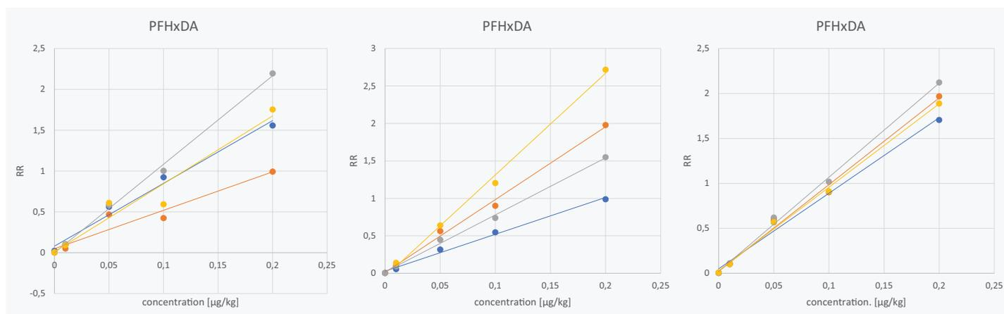
**Figure 7:** Comparison of relative response versus concentration for PFHxDA in solvent-based standard (blue), egg (orange), meat (grey) and fish (yellow) with direct injection (left), online SPE without cartridge wash (middle) and online SPE with cartridge wash (right).
