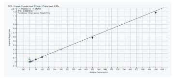
**Figure 3:** Representative calibration curve for extracted BPA standards.
