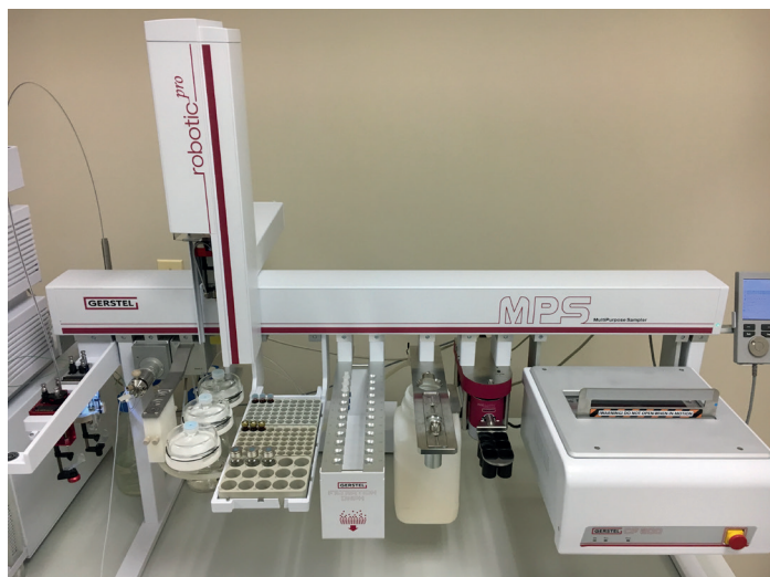
Figure 1: GERSTEL MPS robotic PRO sampler with Agilent LC System. The MPS is configured with Filtration Option, which was not used in this work.
