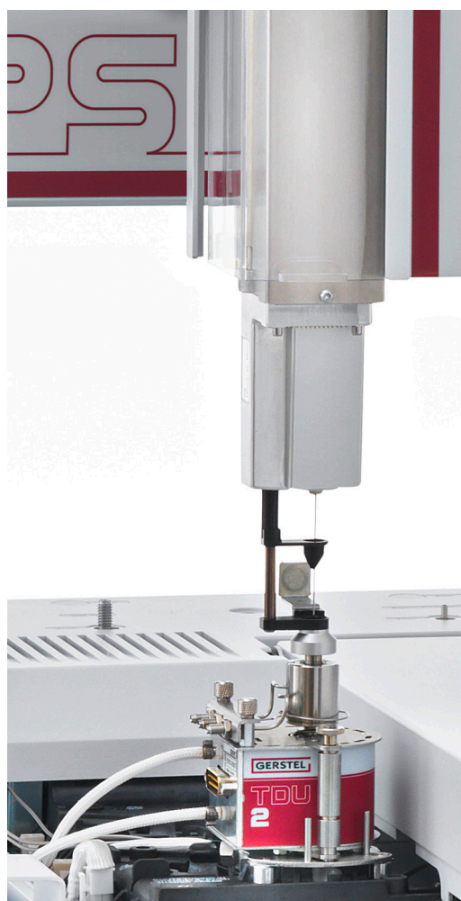
Figure 1: Static headspace injection into the TDU 2 in HIT-HS mode.
