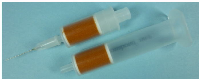
Figure 2: Top: Solid phase extraction cartridge configured for automated GERSTEL SPE. Bottom: Standard solid phase extraction cartridge.
