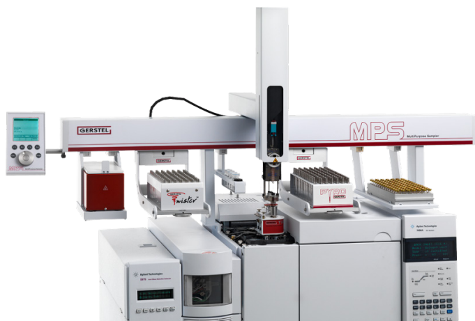
Figure 1a: GC/MS system equipped with a Thermal Desorption Unit (TDU), Pyrolysis Module (PYRO), and MultiPurpose Sampler (MPS) used for automation of all sample introduction techniques.
