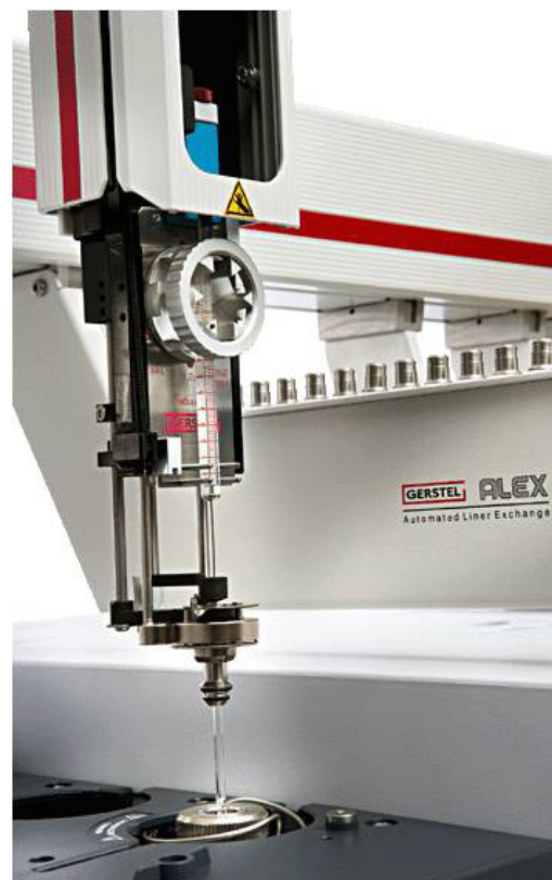
Figure 2: MultiPurpose Sampler (MPS) equipped with gripper for automated liner exchange. The 14-position ALEX liner tray is shown to the right.
