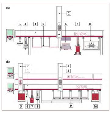
MultiPurpose Sampler (MPS) Systems for automated sample preparation, derivatization of fatty acids from human plasma phospholipid fractions as well as sample introduction to GC/FID.
