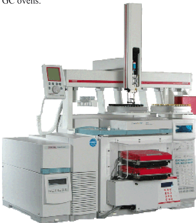
Figure 1. Dual column MACH connected to 6890 GC system.
