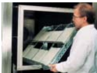
Figure 1 Loading a 1 \text{ m}^3 test chamber with adhesive on glass plates
