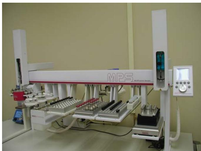
**Figure 1.** GERSTEL MultiPurpose Sampler (MPS) Dual Head WorkStation configured with mVORX, mVAP, and Universal Filtration Options.
