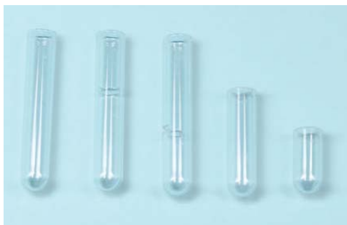
Figure 2. Different microvial designs (from left to right): standard, slit at 1.5 cm from bottom, slit at 1 cm from bottom, cut at 1.5 cm from bottom, cut at 1 cm from bottom. For this study all slitted and cut microvials were produced manually. Currently the left and middle microvials are commercially available (p/n 014756-002-00 and 014756-601-00).
