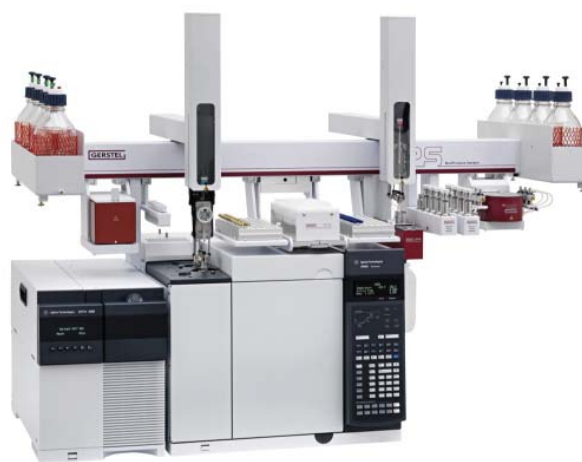
Figure 1. Instrument setup for the automated determination of THC and metabolites in blood serum. Dual Head MultiPurpose Sampler (MPS) equipped with agitator, standard wash station, trays for eluate vials, SPE cartridges and samples, SPE module, two solvent filling stations (SFS), Multi-Position evaporation station (mVAP) and solvent bottle station (from left to right). Left head with 10 \mu L syringe for injection, right head with 2.5 mL syringe for sample preparation steps. GC/MS system: Agilent GC 7890 / MSD 5977 (Agilent Technologies).
