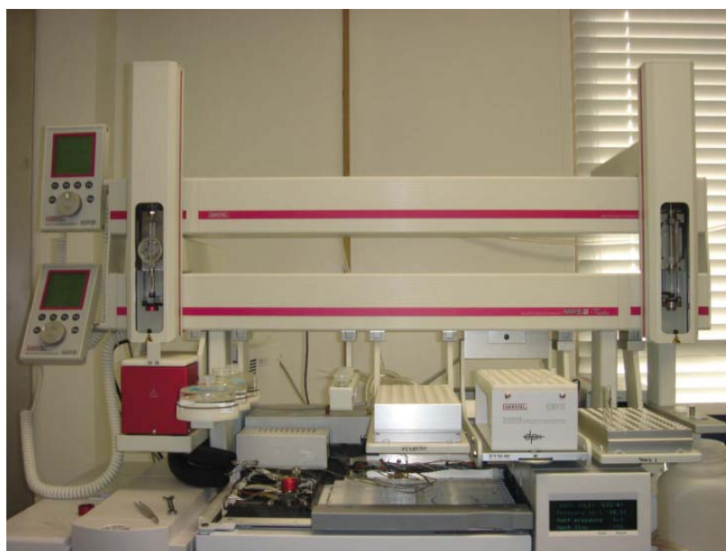
Figure 1. A picture of the dual rail GERSTEL MPS 2 with DPX automation platform. The left MPS is equipped with a 100 µL syringe for injecting eluent and derivatizing reagents, and the right MPS is equipped with a 2.5 mL syringe for performing DPX extractions.
