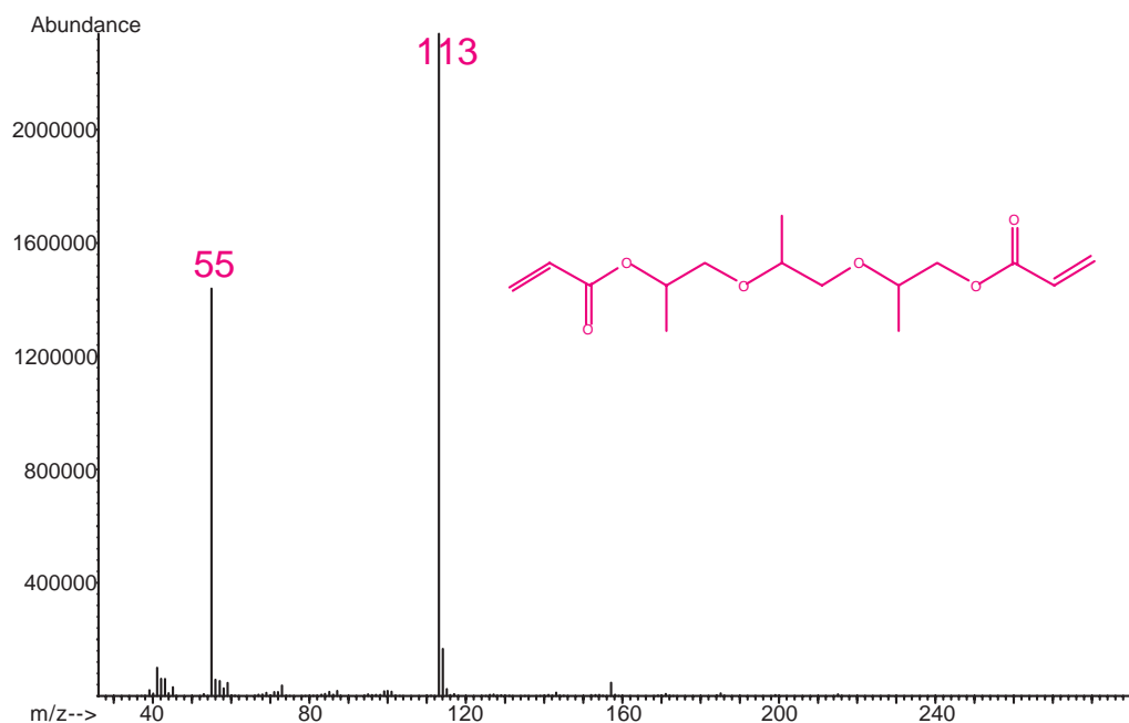
Figure 7. Mass spectrum of tri (propylene glycol) diacrylate (TPGDA).
