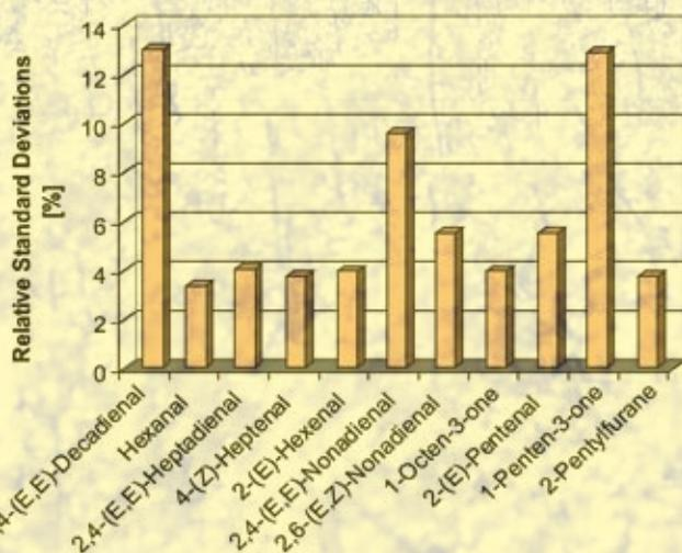
Repeatability was tested with fresh rapeseed oil which had been spiked with 5 ng/g of each analyte. The RSD for five runs was under 6 % for most compounds, this was at least as good as the results obtained when performing the analysis with HS-SPME.
