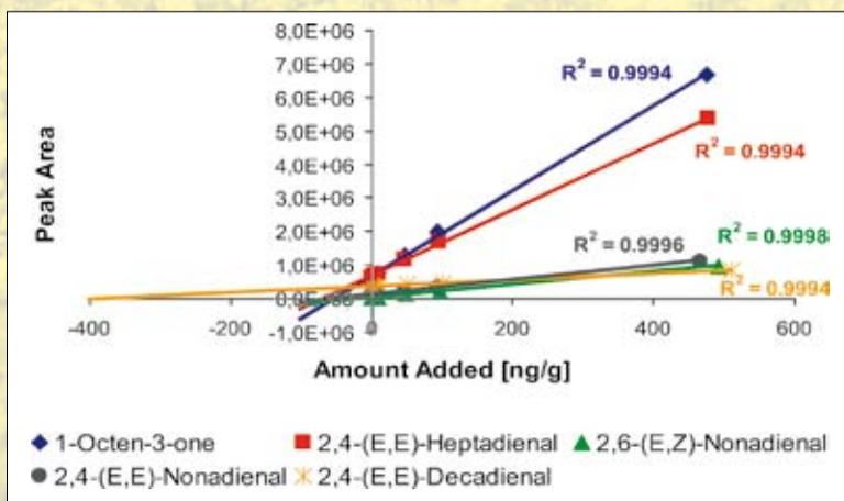
The standard addition calibration curves for the different compounds in an oil sample are linear up to 500 ng/g. The correlation coefficients were around 0.999 for almost all compounds.
