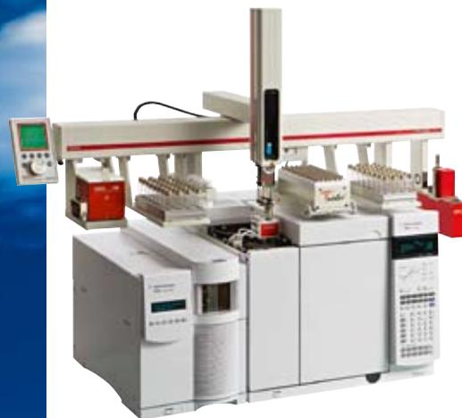
For the determination of quality markers from fatty acid decomposition, the GERSTEL scientists relied on an automated DHS-GC/MS system. The instrument set-up has been implemented successfully for this application in customer laboratories.
