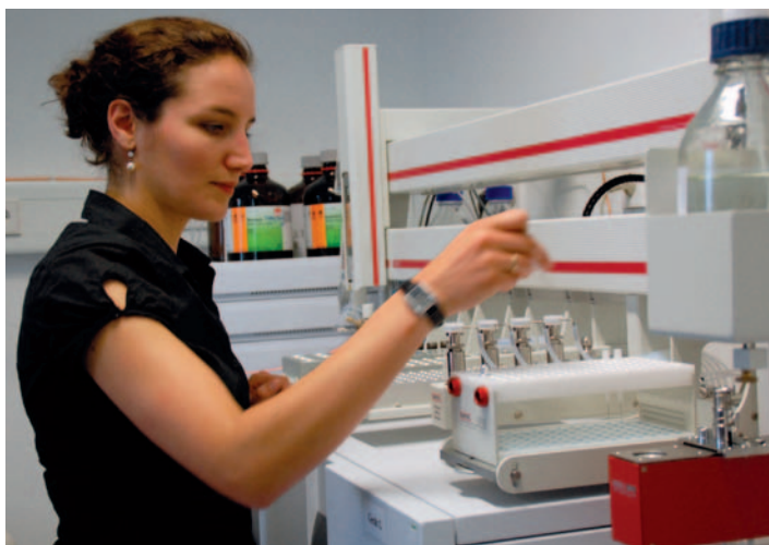
Co-author Meike Baden at the SPE-LC/MS/MS System used for this work. The dual rail MPS enables additional automation of liquid handling steps performed during sample preparation.
