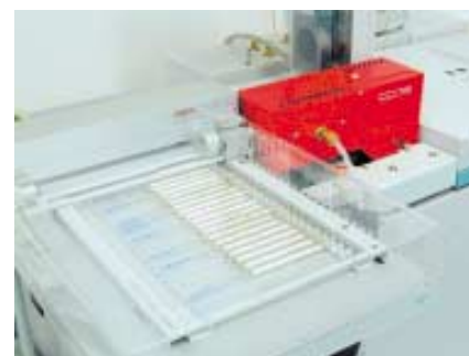
Figure 3 GERSTEL TDS system with autosampler mounted on 6890 GC with 5973 MSD
