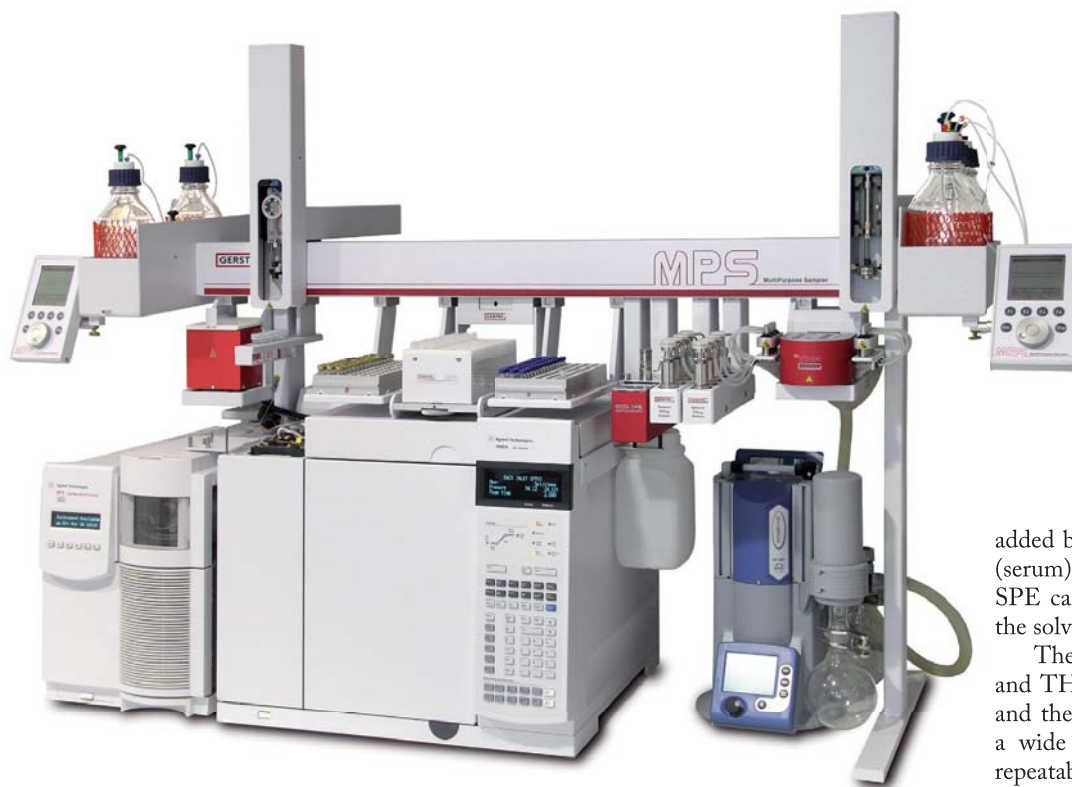
MPS-GC/MSD system used for THC analysis. From the right: Four-position solvent reservoir; multi-Position Evaporation Station (M 2 VAP) for eluate evaporation with the associated vacuum pump placed below; dual Solvent Filling Stations (SFS) supplying large volumes of solvents; SPE station; sample vial tray; SPE cartridge tray; eluate vial tray; Solvent Wash Station for syringe rinsing; Heated Agitator; second solvent reservoir.
