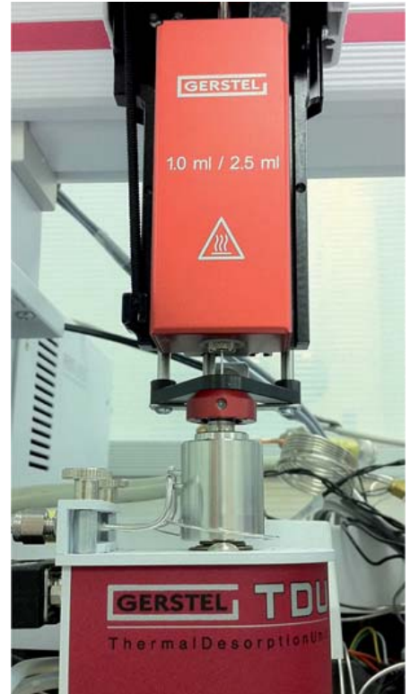
The GERSTEL MPS configured for HIT-SPME in combination with the TDU.
