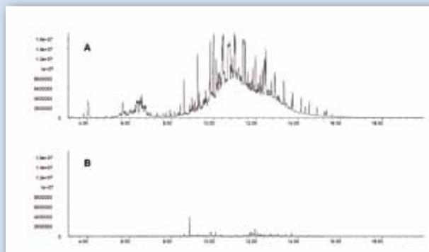
TDS-GC/MS chromatograms of individual parts multicomponent pharmaceutical packaging system as well as an organic extract. It was not possible to identify the compound marked with \* just based on GC/MS.
