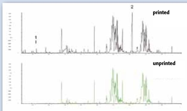
Comparison of two HS-GC/MS chromatograms (SIM mode) of pharmaceutical product stored in A: Polymer packaging material onto which text has been printed; and B: Polymer packaging material onto which no text has been printed. The compound shown is benzene.
