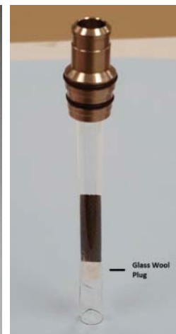
Figure 2. TF-SPME device in TDU tube.
