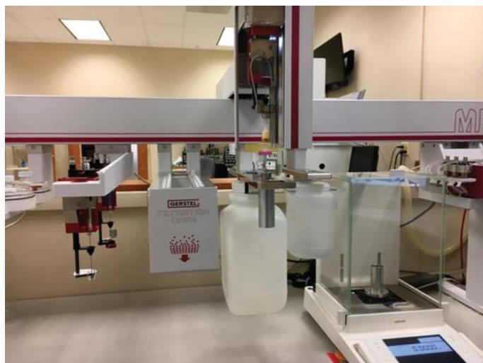
Figure 2. GERSTEL MPS robotic<sup>PRO</sup> sampler with GERSTEL DNPH Option.
