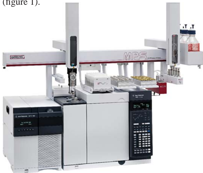
Figure 1. GC/MS system used for automated determination of benzo[a]pyrene and benz[a]anthracene in tar distillation products.
