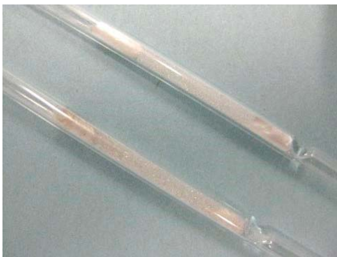
Figure 16. CIS GC inlet liner new (top) and after >50 samples (bottom). Due to effective sample cleanup, the used inlet liner is relatively clean.
